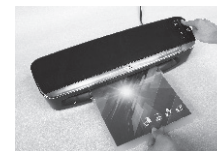
(Fig. 6) In case of pouch jam, press the REV. button and you hear the beeping sound. Pull out the jammed lamination from the Pouch entry .
