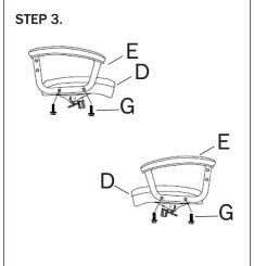
DO NOT fully tighten Screws (G)
