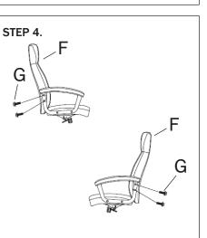
DO NOT fully tighten Screws (G)
